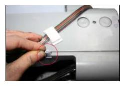
Insert a scrip in the proper position of printer top cover as the picture shown above.
